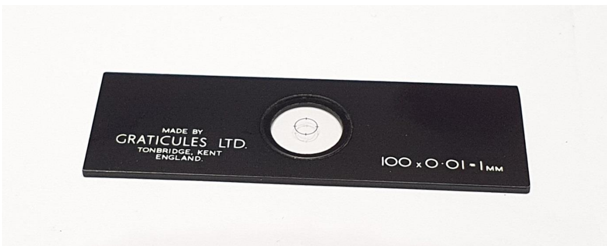
Figure 6. A 1mm stage graticule with 10\mu\text{m} divisions.
