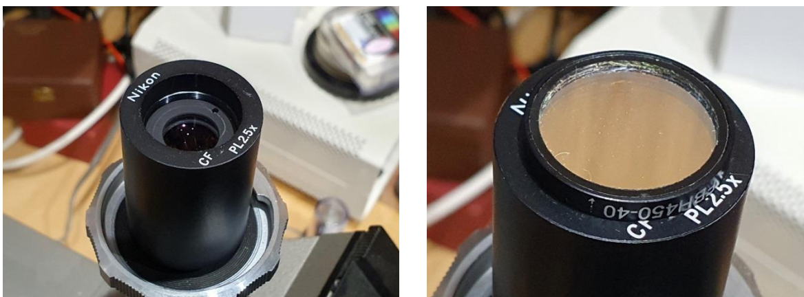
Figure 4. Nikon 2.5x CF PL photoeyepiece (left) and Thorlabs 450nm, 40nm FWHM filter (right).
