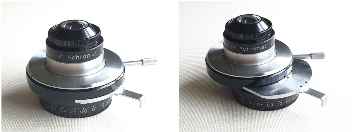
Figure 2. Olympus Aplanat Achromat condenser in standard brightfield configuration (left) and setup of oblique illumination (right).
