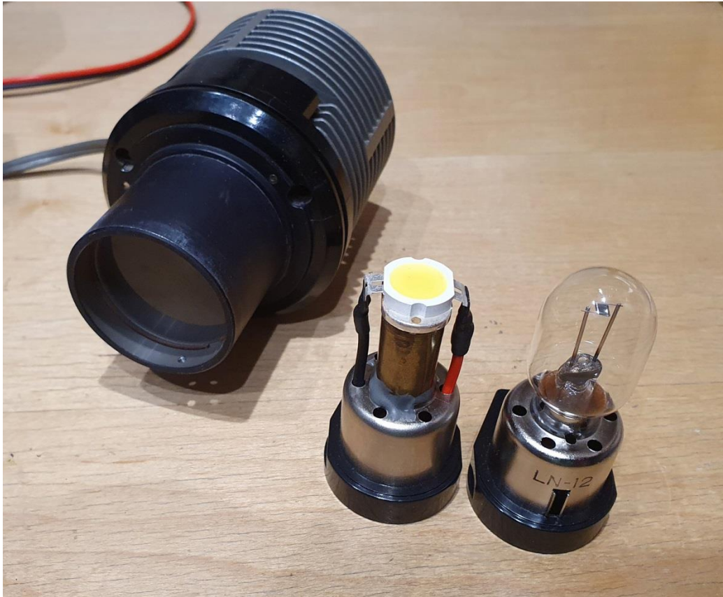
Figure 5. Olympus lamp housing (left), white LED conversion (middle) and original bulb (right).
